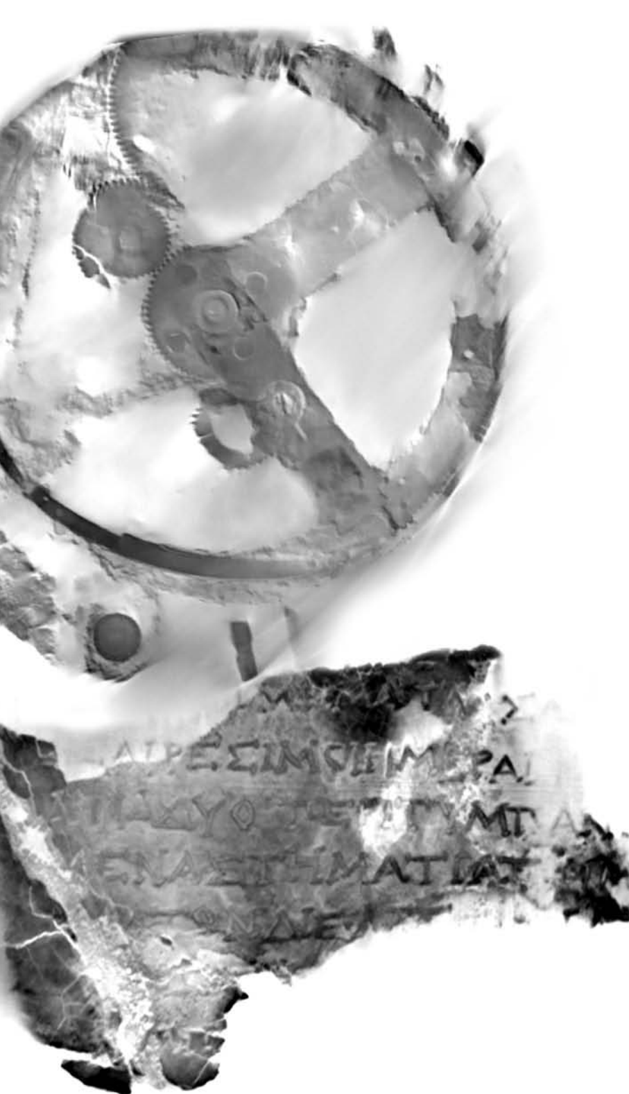
Slices from the computed tomography data showing the inner structure of fragment A and an invisible text inside fragment E (not in scale)
